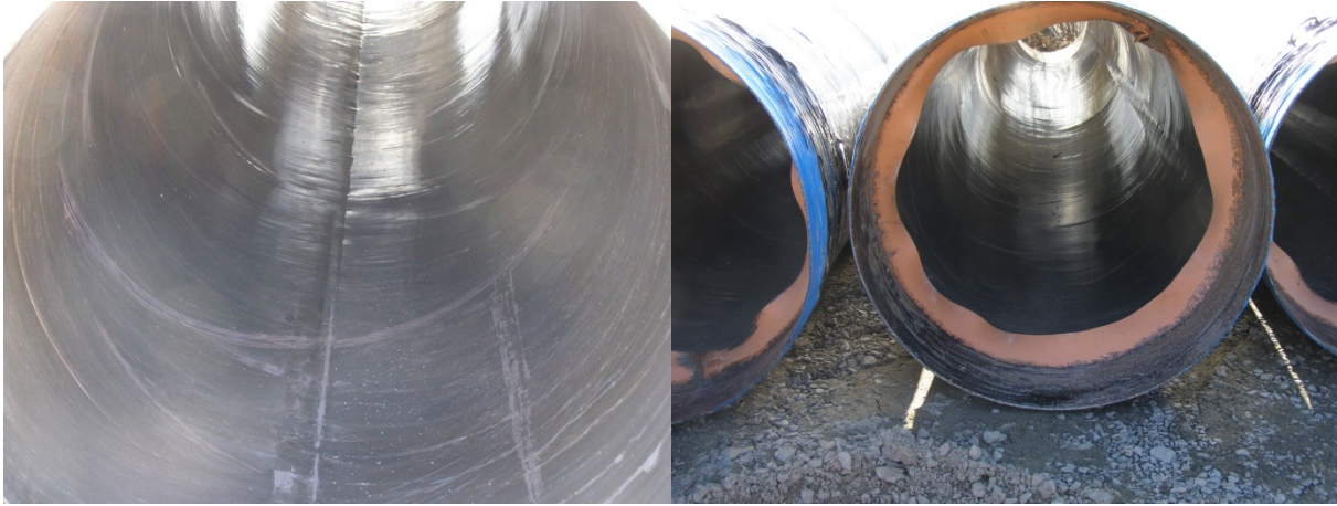
Figure 5 Internal surface of new style manufacture and the rubber sealing gasket
