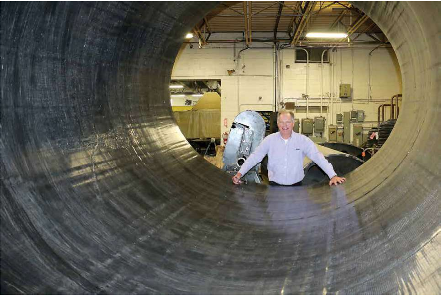
Don Croteau, managing director of Schauburg Industries with massive 2.3-metre diameter section of rigid fiberglass ventilation ducting destined for the Crosslinks light rail transit line along Eglinton Avenue in Toronto.
